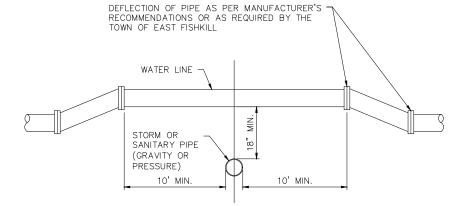
NOTE: FOR ANY CONDITIONS OTHER THAN SHOWN AT THE LEFT, THE FOLLOWING REQUIREMENTS SHALL BE MET: THE JOINTS OF THE SANITARY SEWER OR STORM DRAIN SHALL BE A MINIMUM OF 10' FROM THE POINT OF CROSSING. THE SANITARY SEWER SHALL BE CLASS 150 PRESSURE PIPE AND THE STORM DRAIN SHALL BE LOCK-JOINT PRESSURE PIPE. WHERE THE ABOVE CONDITIONS CANNOT BE MET, THE DUTCHESS COUNTY DEPARTMENT OF HEALTH SHALL BE NOTIFIED AND THEIR APPROVAL SHALL BE REQUIRED.
