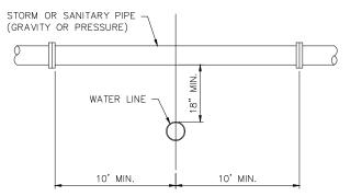
NOTE: WHERE THE WATER LINE PASSES BENEATH THE SEWER LINE OR STORM DRAIN, THE JOINTS OF THE PIPE SHALL BE A MINIMUM OF 10' FROM THE POINT OF CROSSING. SEWER PIPE SHALL BE CLASS 150 PRESSURE PIPE AND THE STORM DRAIN SHALL BE LOCK-JOINT PRESSURE PIPE.
